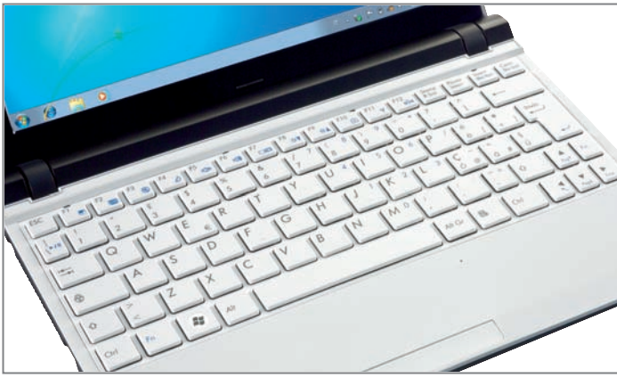
ERGONOMIC KEYBOARD with an island layout where the keys are each separated from each other
